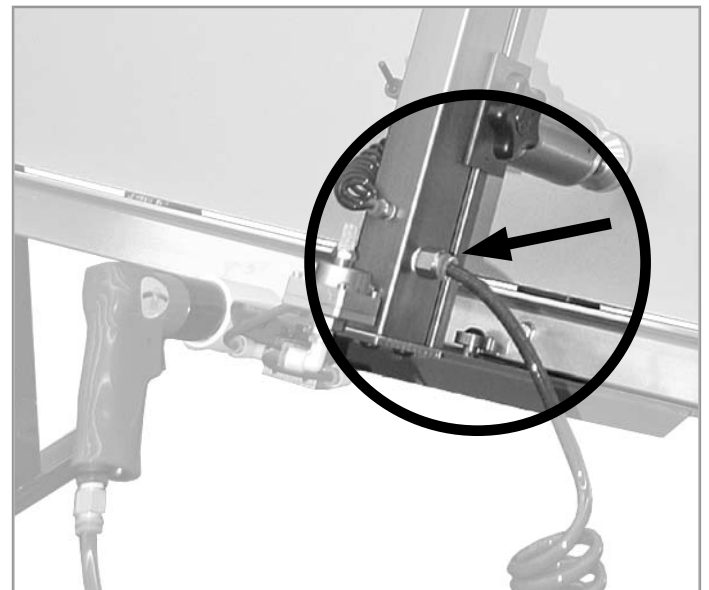
Hose and gun attached to the main rail.
